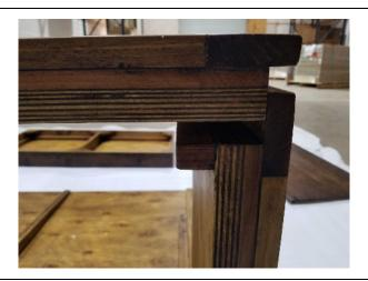
2a) Attached front panel by sliding in place as shown.
